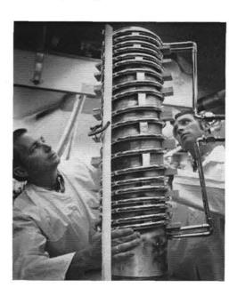
INDUCTION HEATING COIL is readied by Dick Curlee, left, and Don Cook of the Carbon Processing Laboratory 5312 before installation in a furnace.
